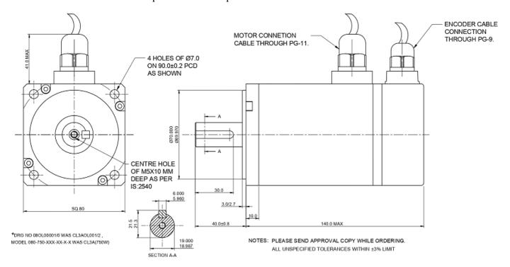
750 Watts Motor without brake
