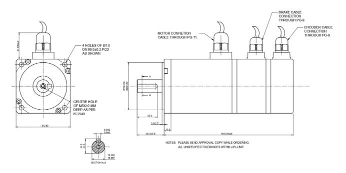
750 Watts Motors with brake
